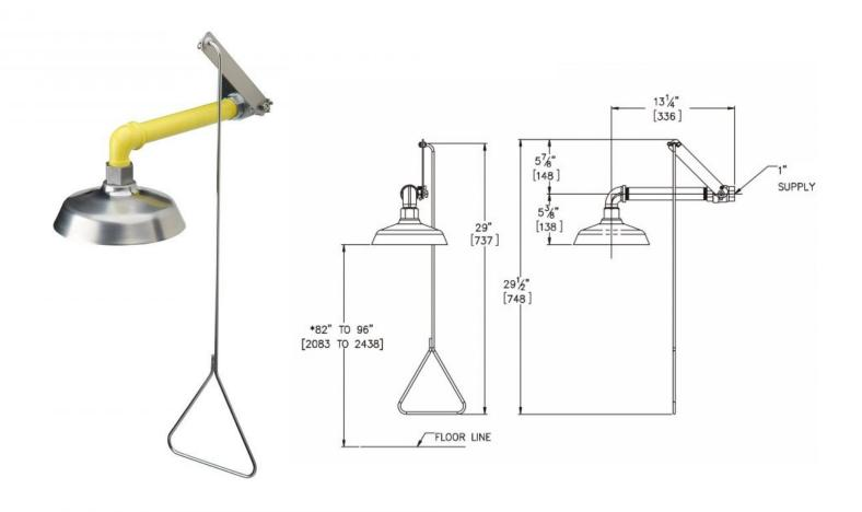
Model S2200 is our horizontal wall mounted safety shower with stainless steel head. Supplied with stainless steel pull handle and 1" chrome plated brass stay open ball valve.
